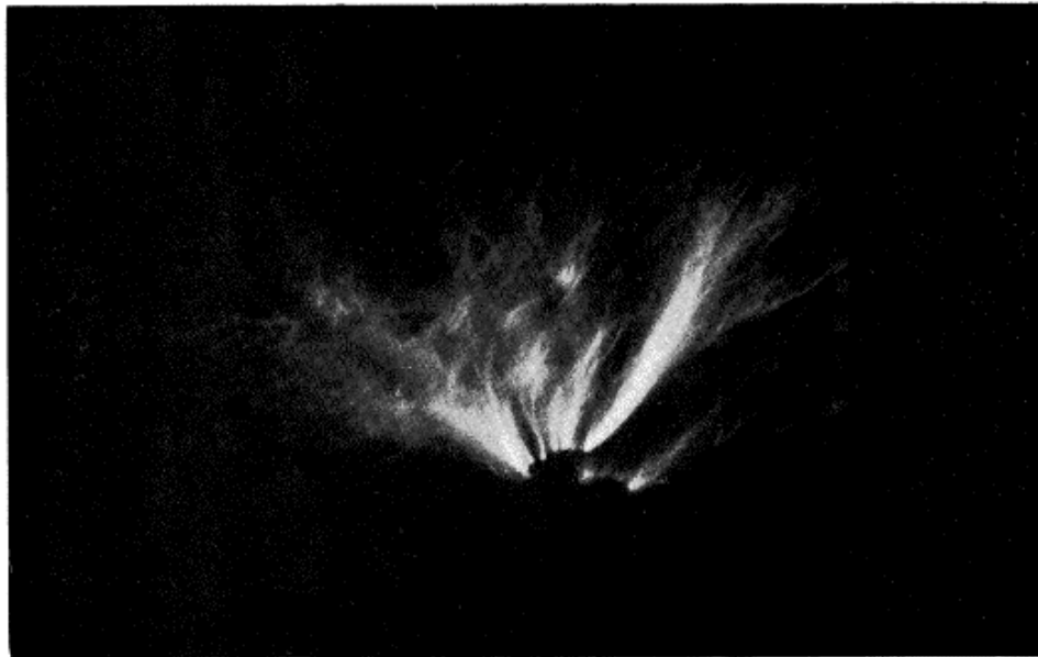
FIG. 14. EFFECT OF ELECTRICAL DISCHARGE FROM THE EARTH BY TESLA COIL. (PHOTOGRAPHED BY ITS OWN LIGHT.)
